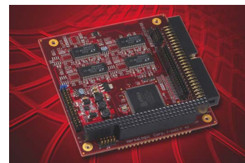
The PC/104 VCM-DAS-3 module features 16 channels of 12-bit analog output and 24 digital-I/O lines to support many embedded-computing applications.
